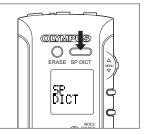
For optimum results in voice recognition and voice-text conversion, press the DICTATION MODE button ③. All settings are automatically adjusted to ensure best results.
